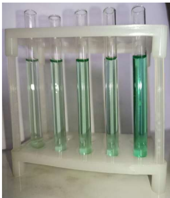
Figure 6. Nickel extraction into solutions of sulfuric acid at different concentrations.
