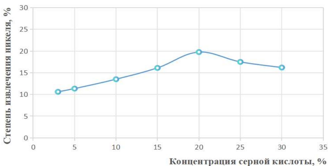
Figure 4. Effect of sulfuric acid concentration on the degree of nickel extraction (S:L = 1:3, temperature 30 °C, n = 500 rpm, \tau = 15 min)
