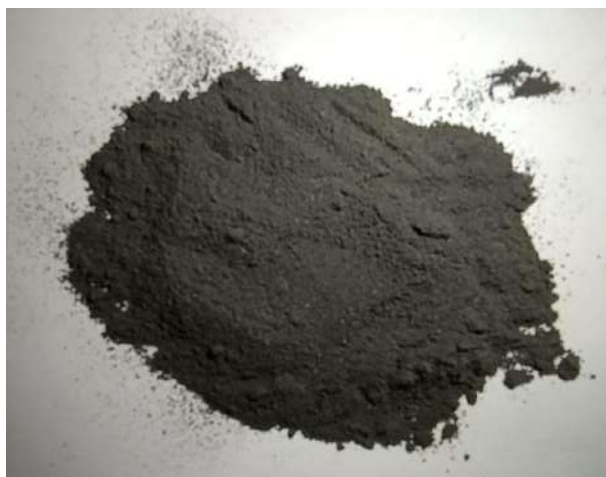
Figure 3. Ground state of the spent hydrogenation catalyst
