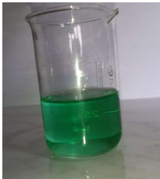
Figure 7. Nickel extraction into a 20% sulfuric acid solution under optimal conditions.
