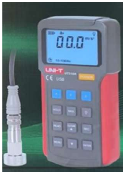
Figure 1. Instrument for measuring rotational self-oscillations
