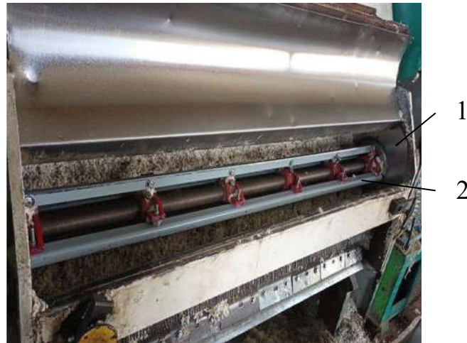
Figure 2. The working chamber of the 5LP linter with improved mixing blades 1- working chamber, 2- improved paddle mixer.
