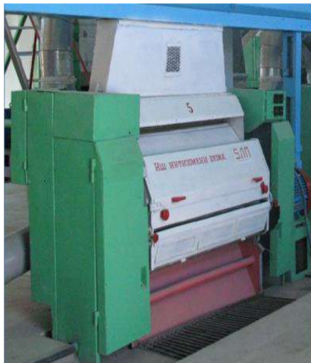
Figure 3. A view of the 5LP linter in production, with blades having an improved agitator
