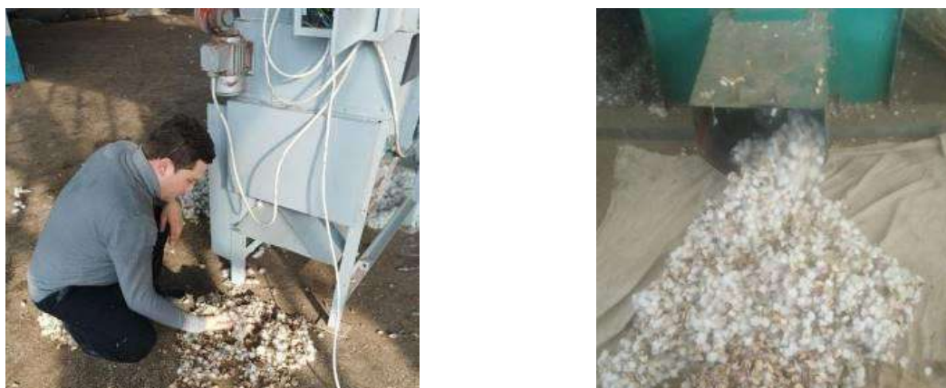
Figure 4. a – large impurities discharged from the device with improved rib design; b – large impurities discharged from the UXK unit.
