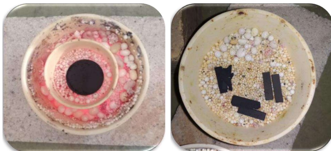
Figure 2. The samples, pressed into a disk and beam, were placed in a crucible filled with corundum spheres
