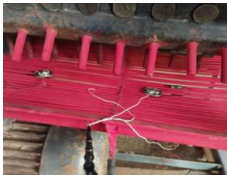
Figure 2. A view of the device with strain gauges installed on the wires
