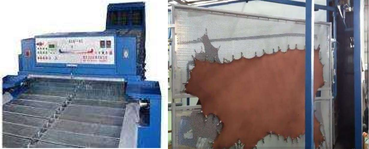
Figure 1 shows the drying of skins under uniform conditions, which allows for the expansion of the drying area of the skins with the help of steam and wind
