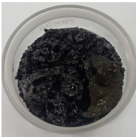
Figure 1. Tar product subjected to thermal activation at 600^\circ\text{C} for 2 hours under an inert (oxygen-free) atmosphere
