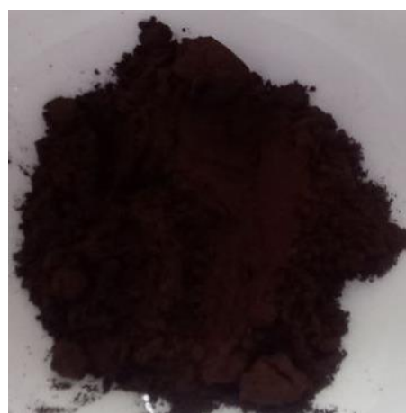
b) Tar product ground to a particle size of 0.071 mm
