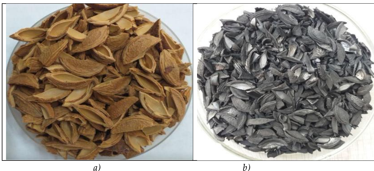
Figure 4. a) plum kernel peel; b) carbonization of plum seed husk
