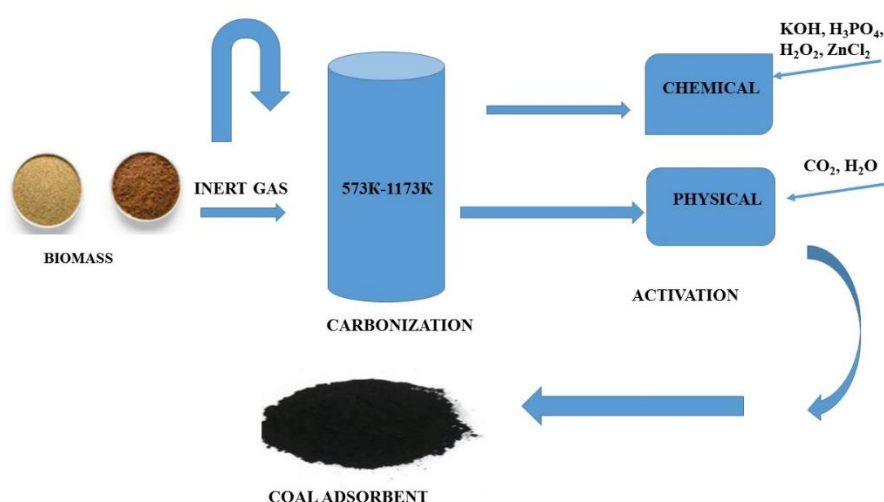
Figure 1. Conventional schematic diagram for obtaining coal-based adsorbents from plant biomass
