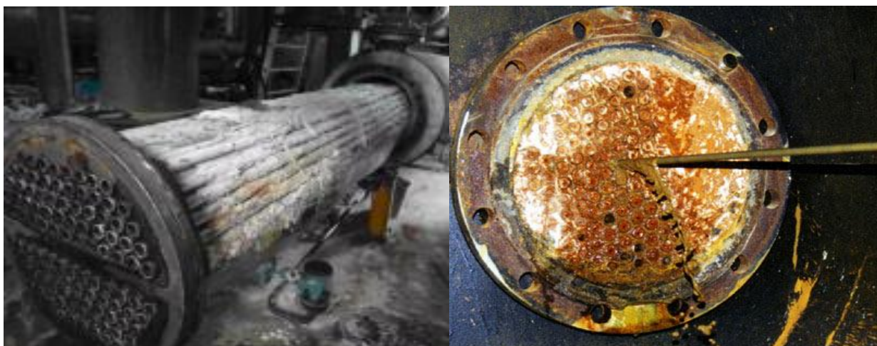
Figure 1. Shell-and-tube heat exchanger and the appearance of the formed scale layer
