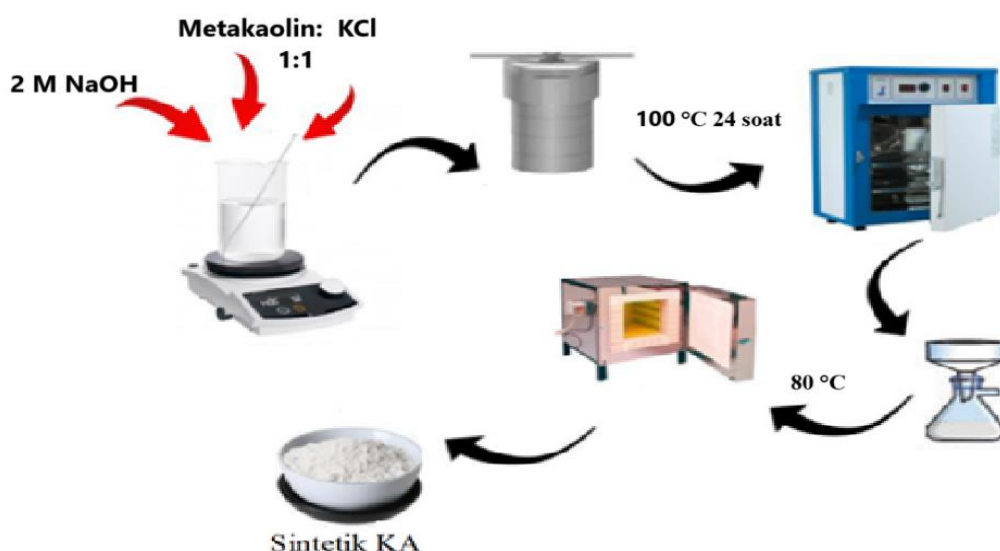
Figure 1. Synthesis diagram of KA zeolite obtained by hydrothermal method
