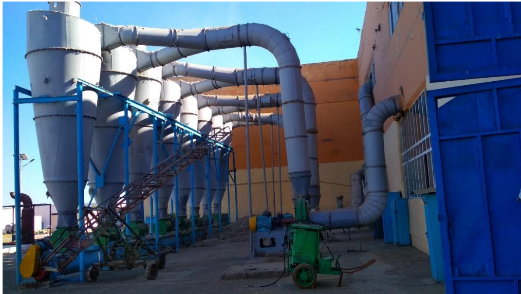
Figure 1. Mechatronic system for cleaning the atmospheric air from dust particles in cotton ginning plants.
