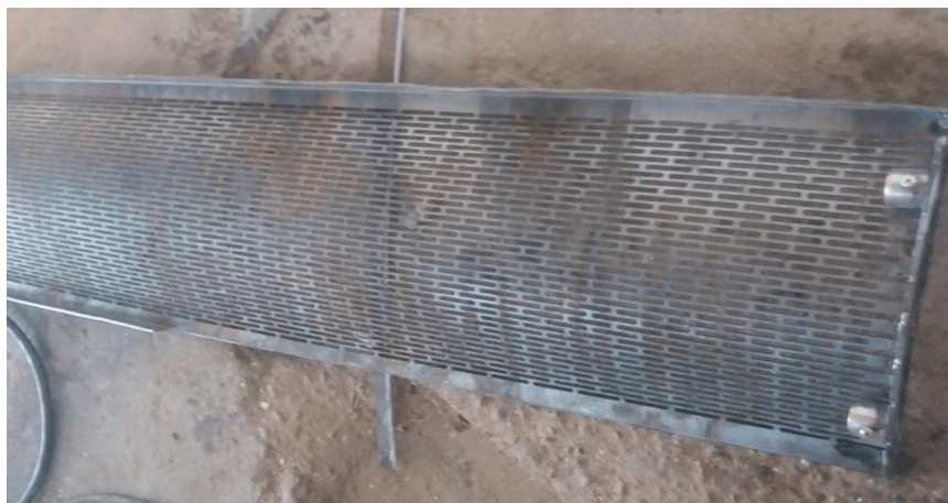
Figure 3.3. Mesh surface for lint removal
