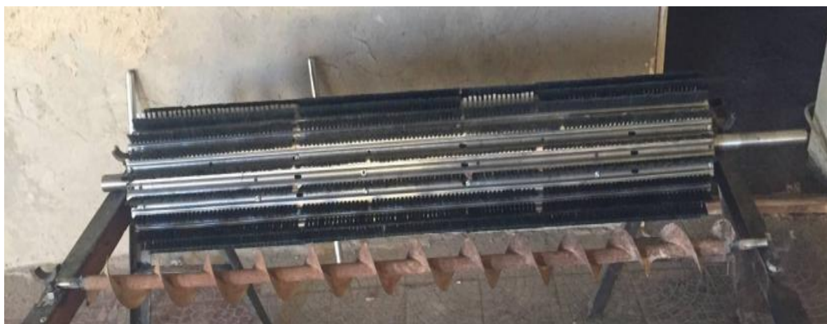
Figure 3.4. Brush drum and dirt auger
