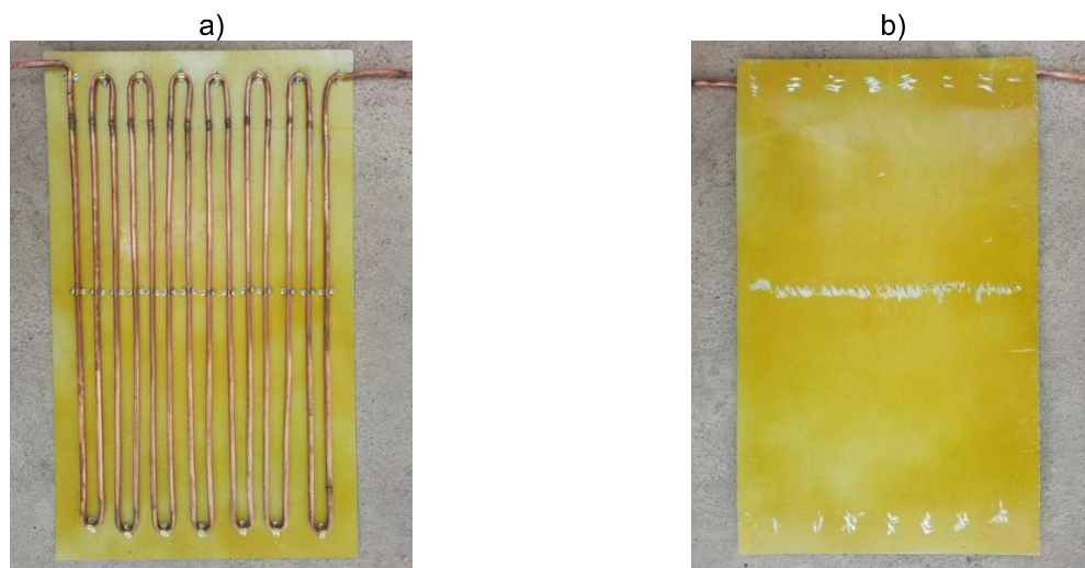
Figure 1. General view of the studied thermal absorber: lower (a) and upper (b) sides
