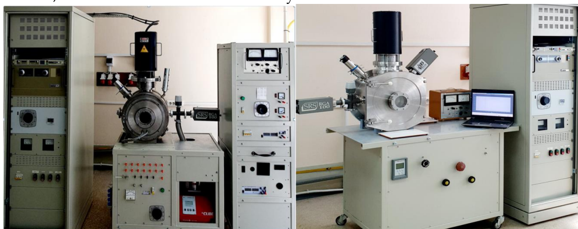
Fig. 1. Coating setup (left), nitriding setup (right).
