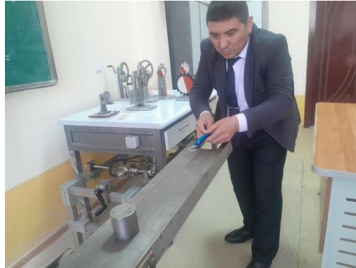
Figure 4. Process of determining static and kinetic friction.
