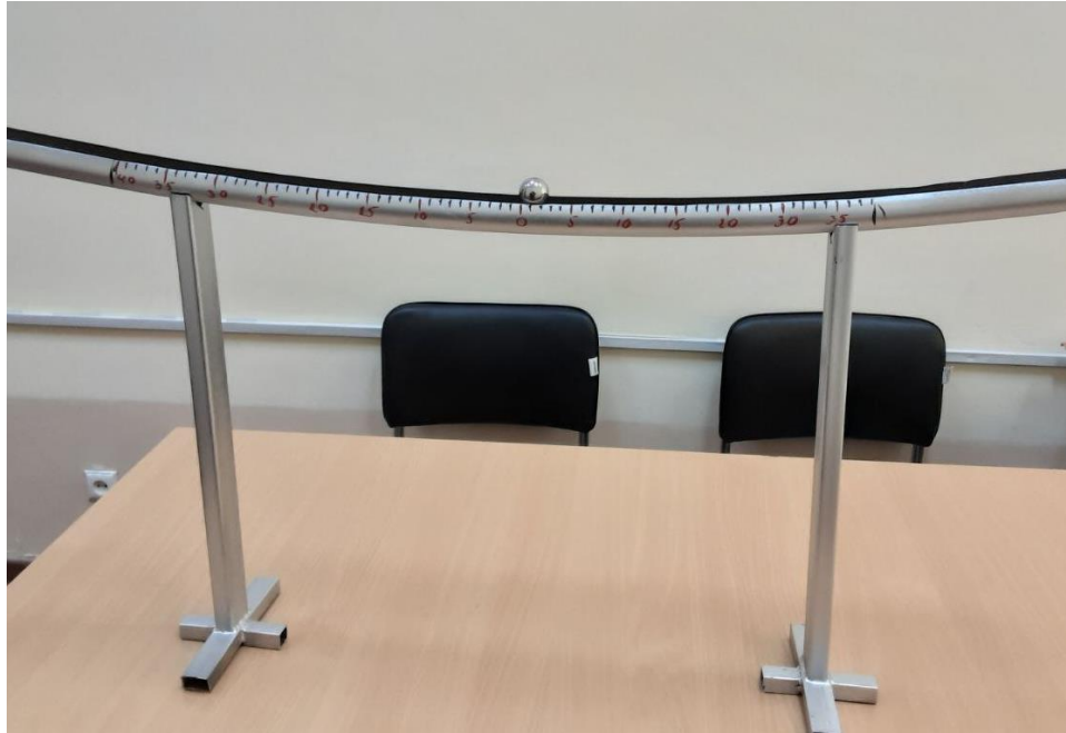
Figure 9. A device for determining the coefficient of rolling friction.
