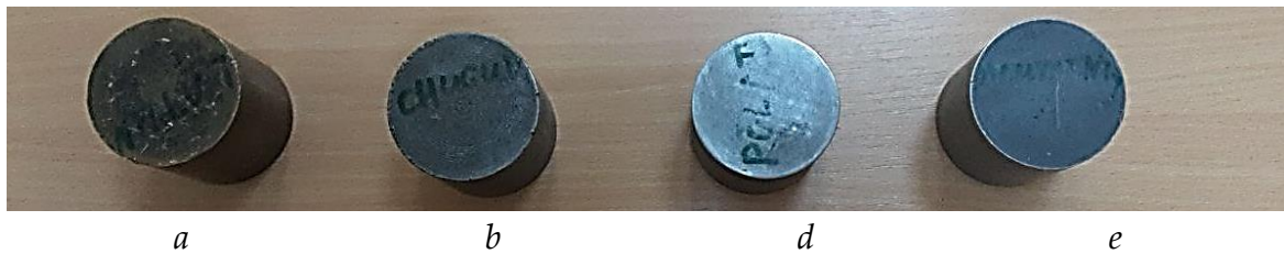
Figure 3. Slippery materials: a- copper , b- cast iron , d- steel , e- aluminum
