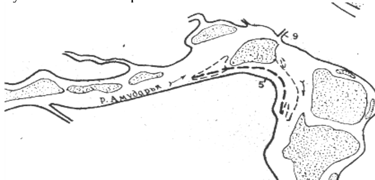
Picture 2. Taking water from the Amudarya River to the Qilichniyazboy Canal and measures to control the river banks
