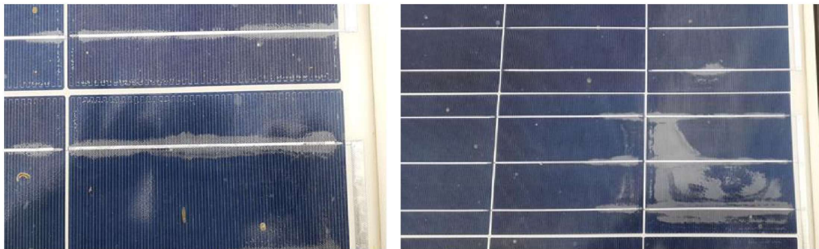
Figure 2. HSL250 defective solar panels from HANHWA
