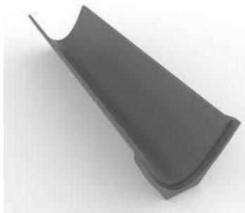
Figure 4. Proposed parabolic elbow view.
