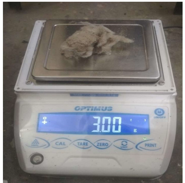
Figure 2 shows the results of measuring fiber waste from the Andijan-35 cotton separator cyclone
