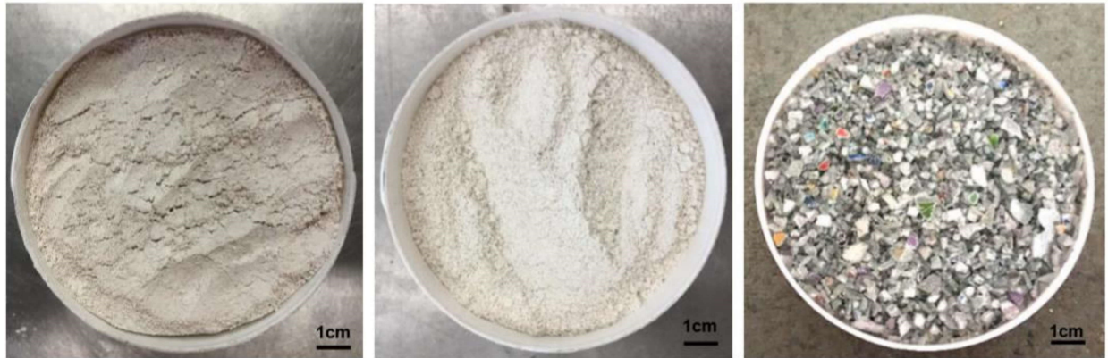
Figure 1. Materials used for the production of new plasters: (a) commercial gypsum; b) unheated gypsum waste from plasterboard production; (c) Polycarbonate waste
