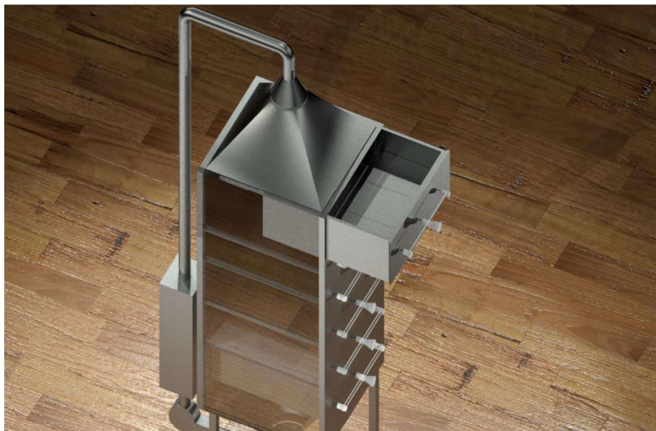
Figure 3. Device for continuous drying of fruits and vegetables
