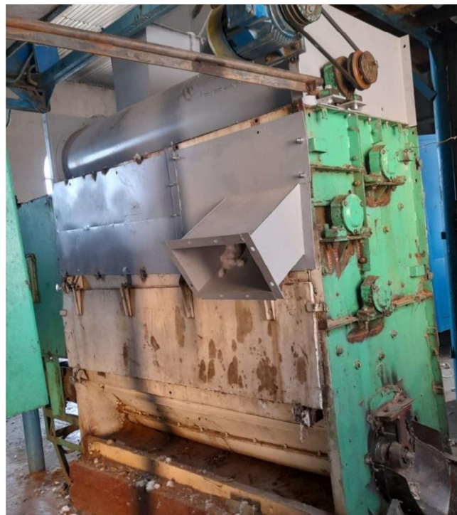
Figure 1. Overview of the improved cotton regenerator
