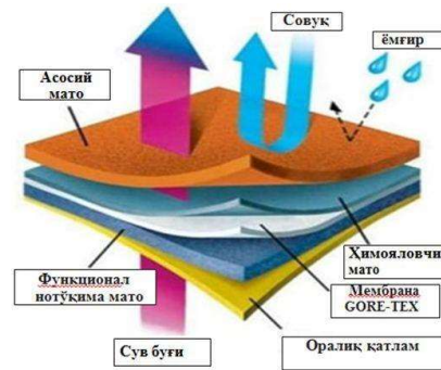
Figure 2. The structure of Gore-Tex fabric
