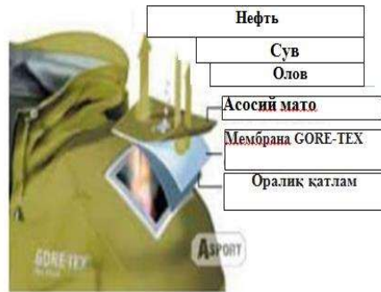
Figure 1. Gore-Tex 2.5. Fabric structure
