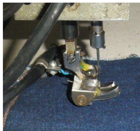
b-paws with load change sensor
