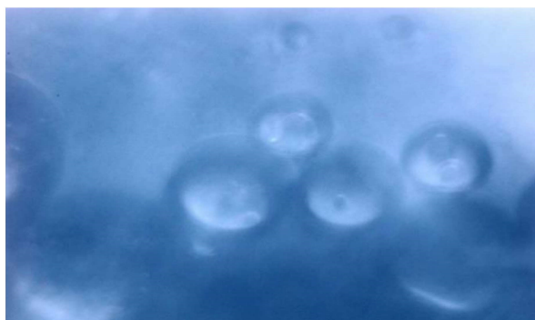
Fig.1 Below is a microscope view of the emulsion obtained through a magnetic stirrer device
