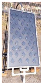
Figure 1.8. External view of the solar air heater
