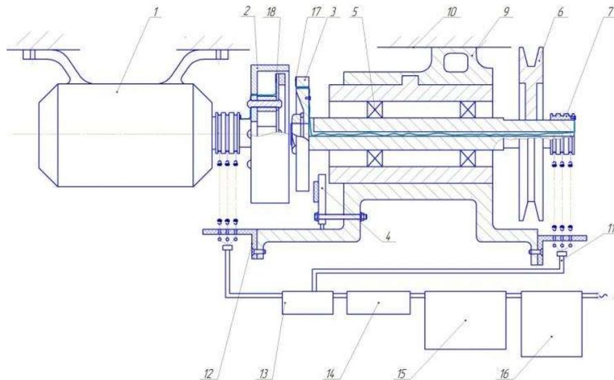
**Fig.3. Scheme of the experimental setup for measuring the torque on the drive clutch of the sewing machine**
