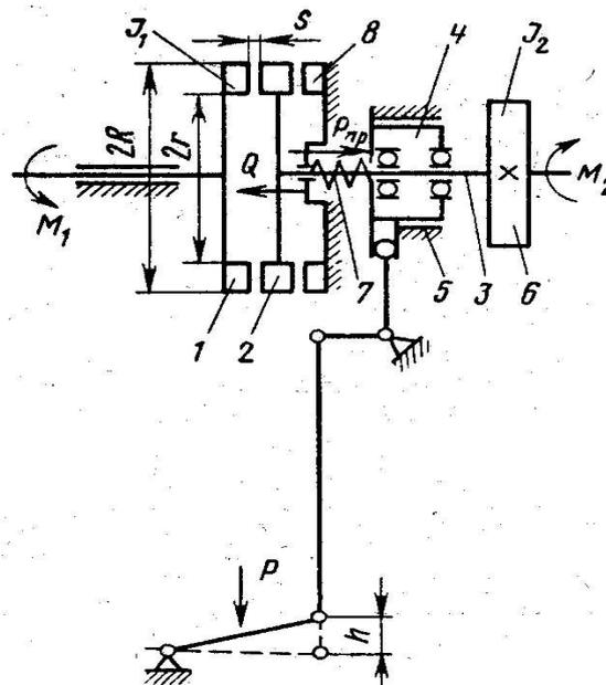
**Fig.1. Kinematic diagram of the friction clutch of the sewing machine drive**
