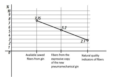
It is known that the percentage of short fibers in fibers is understood to be those that are shorter than 0.5 inches (12.7 mm) in length. Such fibers do not reach in the combing machine, that is, these short fibers do not reach the spinning machine.
