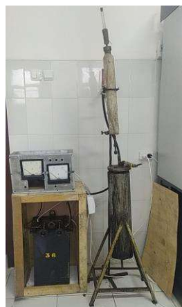
Figure 1. Laboratory plant for the production of activated carbons from organic raw materials
